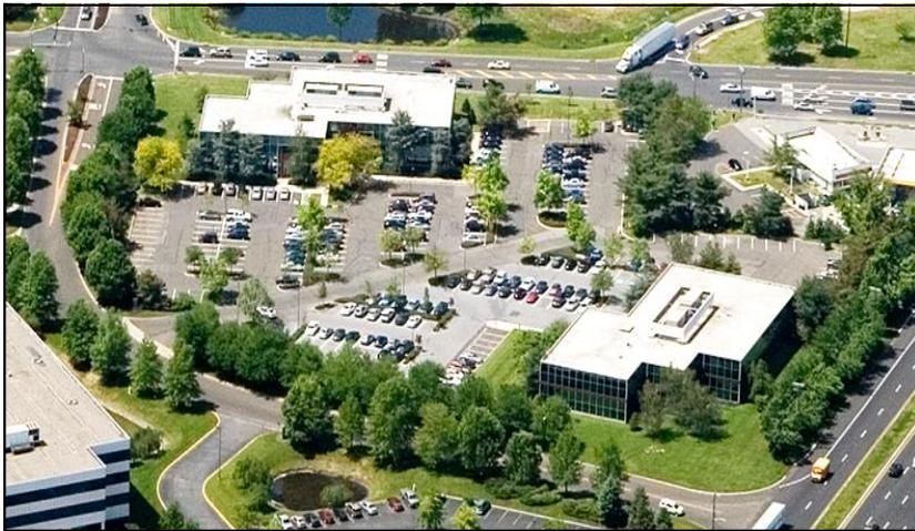
**Roof:** TPO roofs were recently installed at each building. The white roofs reduce solar heat gain due to their reflective qualities which subsequently increases HVAC energy efficiency.
